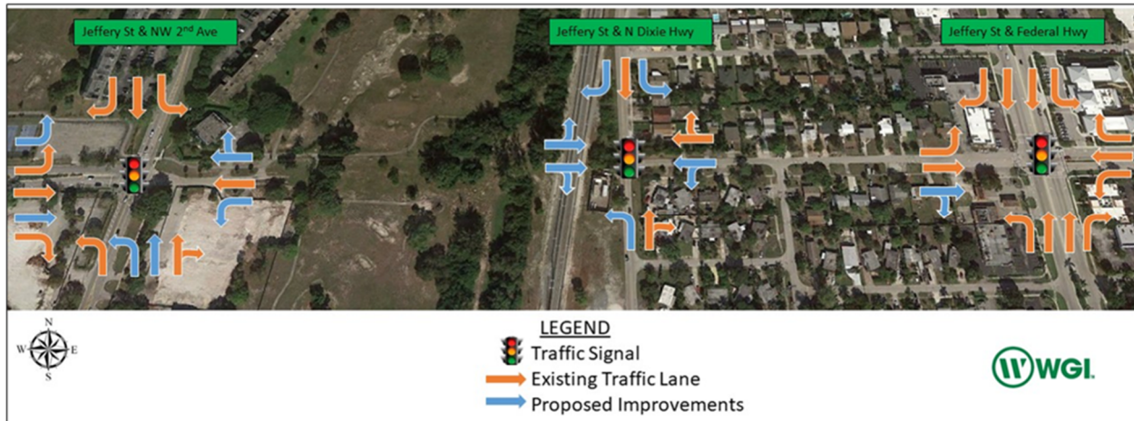
Figure 8: Visual Representation of Mitigations on Jeffery Street
